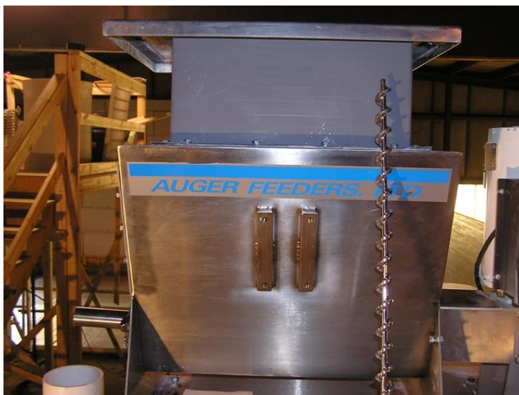
Figure 9: Photograph Showing Variable-speed Auger Feeder
