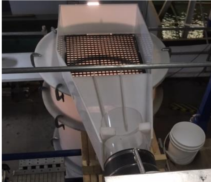
Figure 3: Test Loop Grated Inlet
