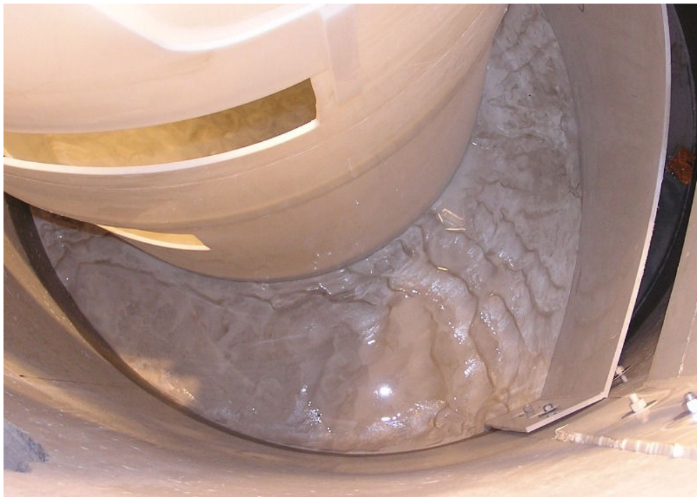
Figure 21: 100% Sediment Bed After Re-entrainment Testing – Middle Chamber
