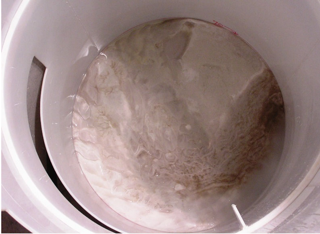
Figure 20: 100% Sediment Bed After Re-entrainment Testing – Inner Chamber
