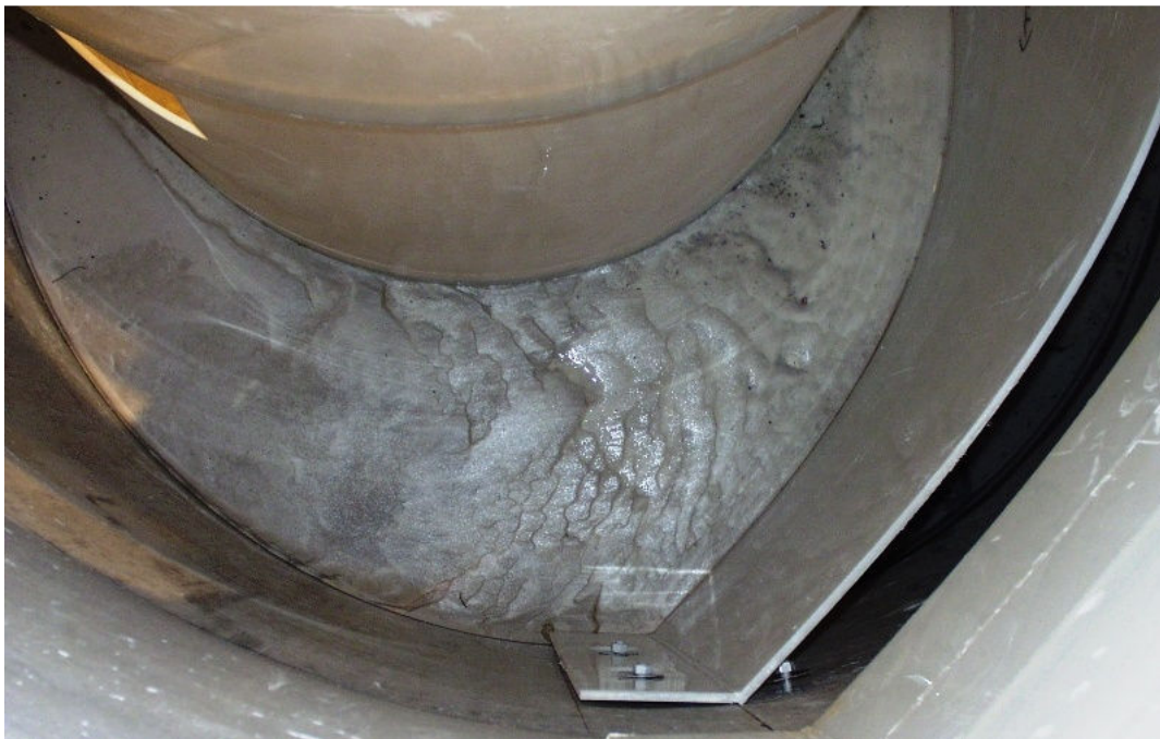
Figure 16: 50% Sediment Bed After Re-entrainment Testing – Middle Chamber
