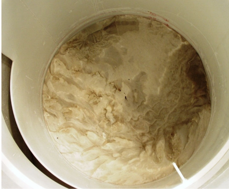
Figure 15: 50% Sediment Bed After Re-entrainment Testing – Inner Chamber
