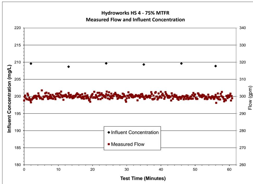
**Figure 14: 75% MTRF Measured Flow and Influent Concentrations**
