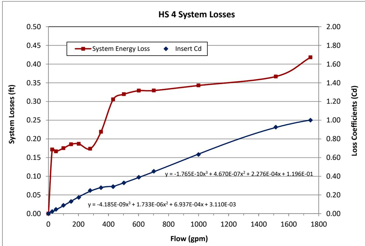
Figure 24: Calculated Losses and Insert Outlet Cd
