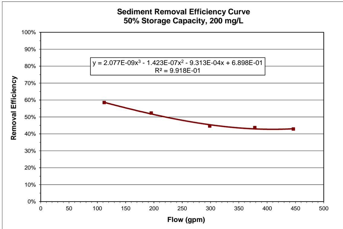
**Figure 9: Hydroworks HS 4 Removal Efficiency Curve**
