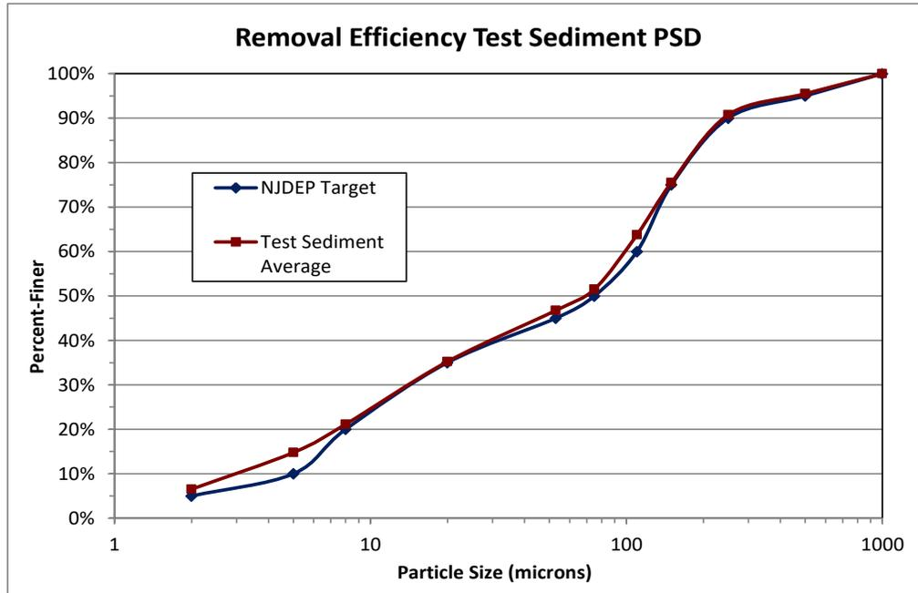
Figure 8: Average Removal Efficiency Test Sediment PSD
