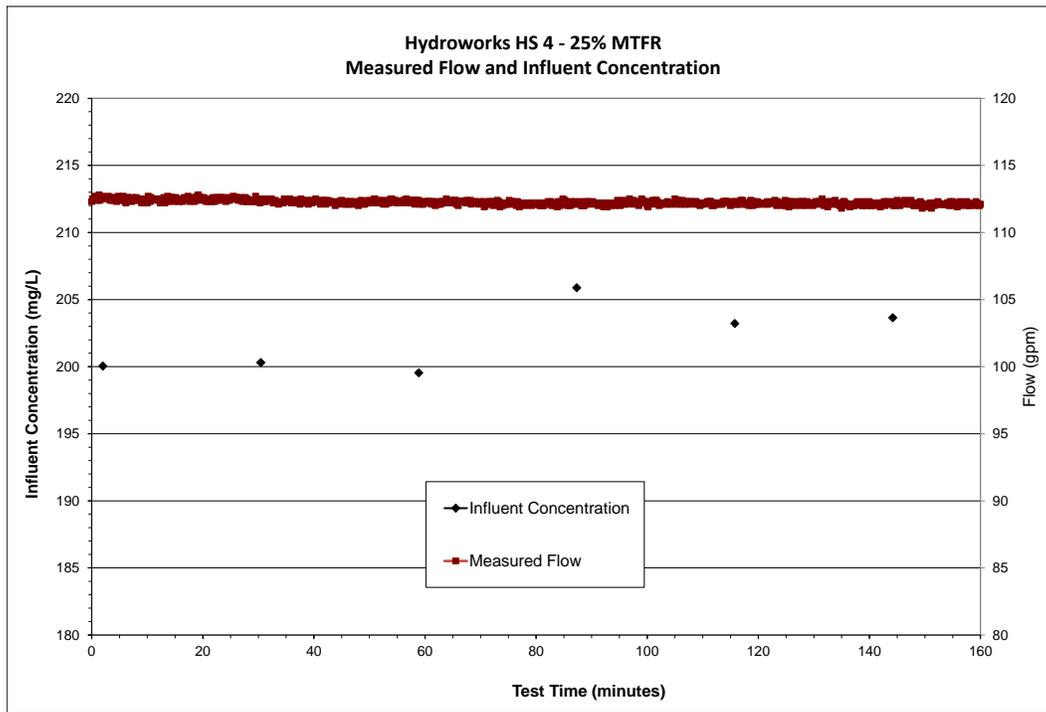
**Figure 10: 25% MTFR Measured Flow and Influent Concentrations**
