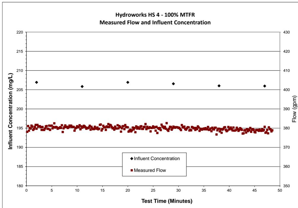
**Figure 16: 100% MFR Measured Flow and Influent Concentrations**
