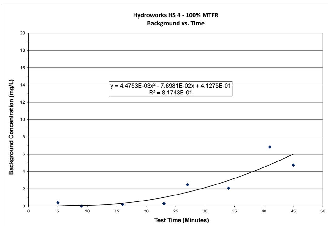
Figure 17: 100% MTR Measured Background Concentrations
