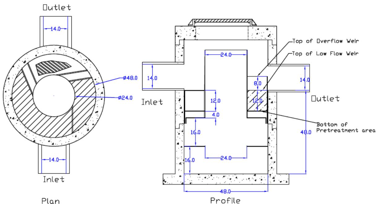
Figure 1: Drawing of the Hydroworks HS 4 Treatment Unit
