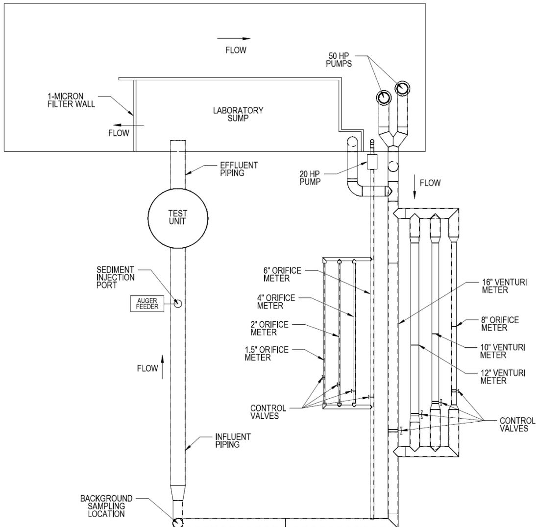
**Figure 3: Plan View of Alden Flow Loop**
