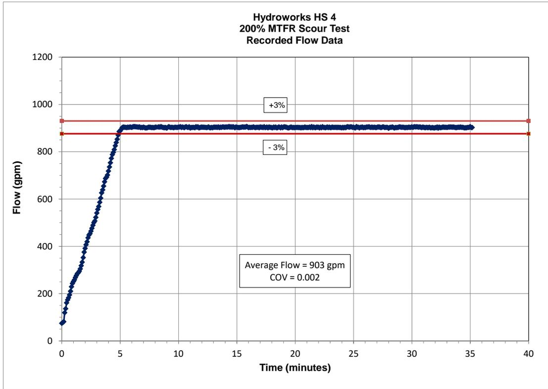
Figure 21: Scour Test Recorded Flow Data
