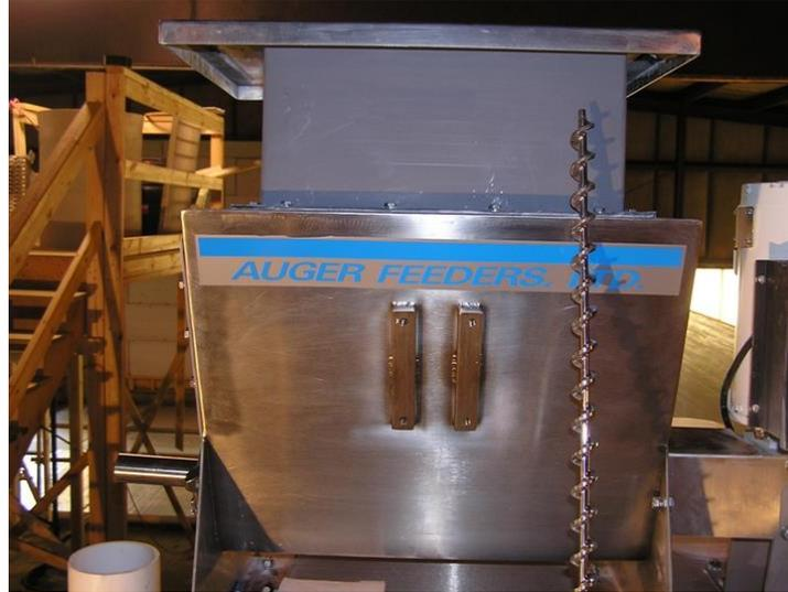
**Figure 6: Photograph Showing Variable-speed Auger Feeder**
