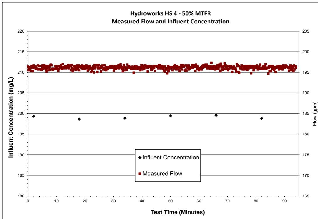
**Figure 12: 50% MTFR Measured Flow and Influent Concentrations**
