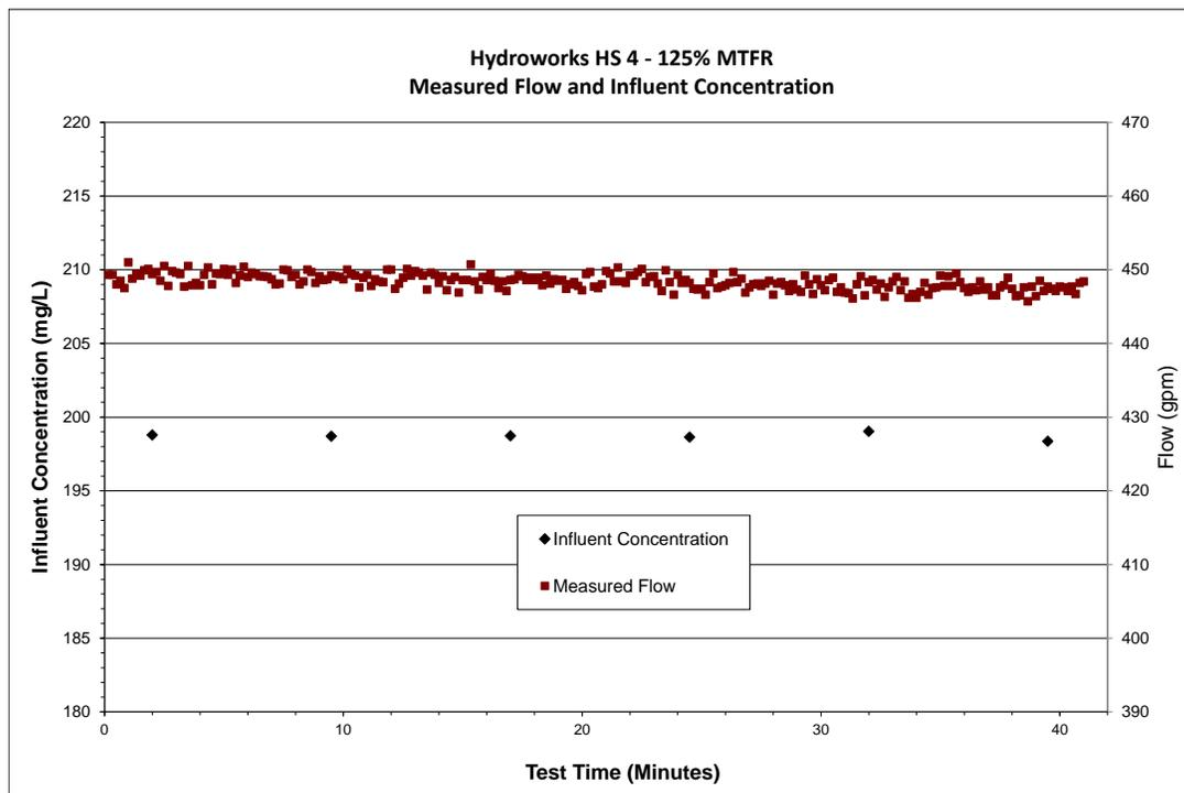
**Figure 18: 125% MTR Measured Flow and Influent Concentrations**
