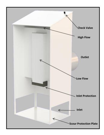
**Figure 2 HydroDome Internal Components**
